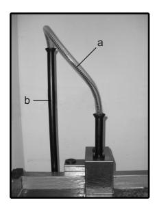
It is important to ensure that the cable conduit (a) can move freely and is not obstructed by other objects.
